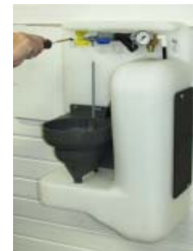
1. Drill holes for the four wall anchors with a (9/32") drill, using the mounting board as a template. Make sure the board is level.
