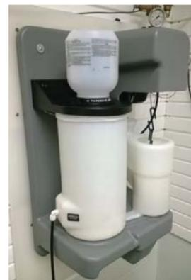
11. Turn the jar 180 degrees to empty the contents into the reservoir.
