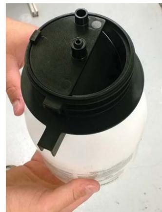
8. Remove the shipping cap and paper seal from the chemical jar.
