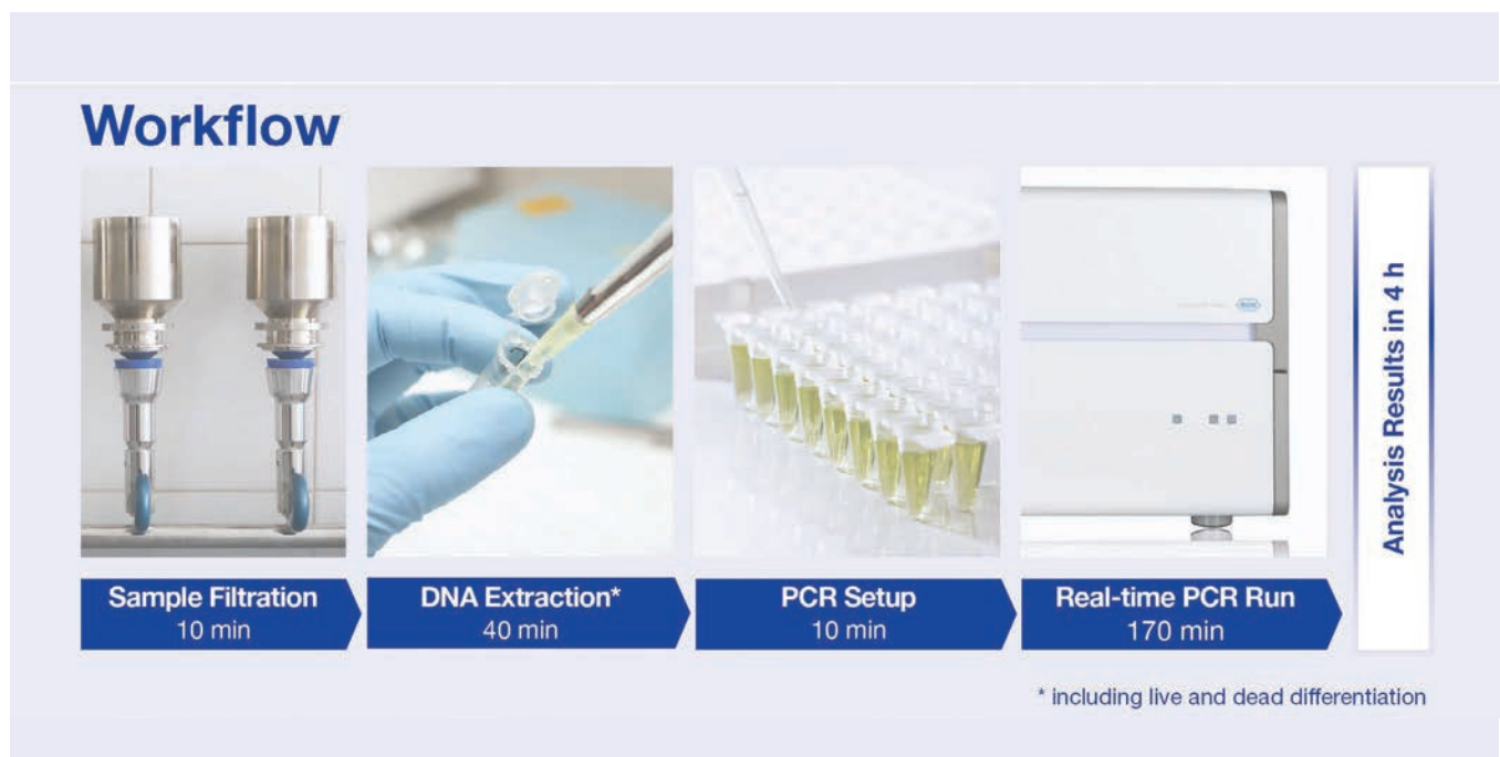
Figure 3: Example test procedure flow and time required for each stage.
